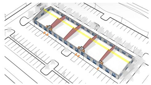
Similar to the baseline design, the NZE Ready design can easily be re-demised over time due to the rhythmic facade. Glazing is optimized - instead of continuous floor to ceiling glazing and ribbon windows, openings are utilized as well as a clerestory (yellow). Each suite can easily have its own entrance.
