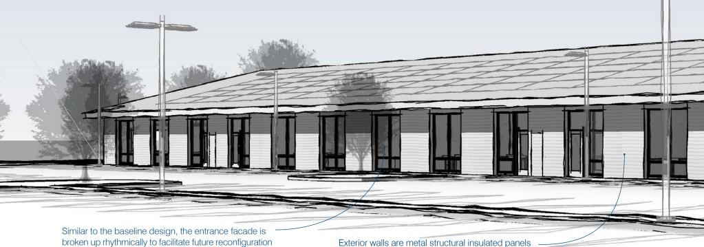
Similar to the baseline design, the entrance facade is broken up rhythmically to facilitate future reconfiguration of space. However, the NZE Ready design has floor to ceiling punched openings with operable windows instead of continuous glazing. This approach optimizes the view and natural light while reducing unwanted heat gain and losses through excess glazing.
